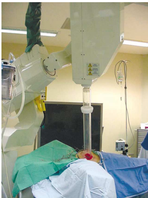
Fig. 1. The dedicated Novac 7 linear accelerator placed in the operating room during a dosimetry procedure. The primary beam stopper and one of the mobile shielding barriers are also shown.
